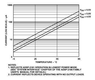
Figure 8. Power-Down Supply Current (Typical)
